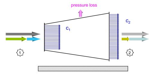
Diffusers are the most efficient way to decelerate air flow, but there'll always be a pressure loss depending on the diffuser design and the inlet conditions
