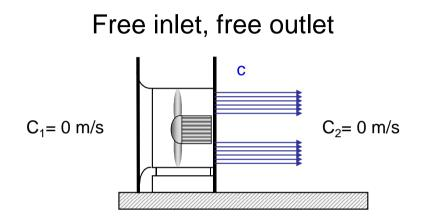
$\Delta p_{\text{static system}} = p_{\text{static fan}}!!$
