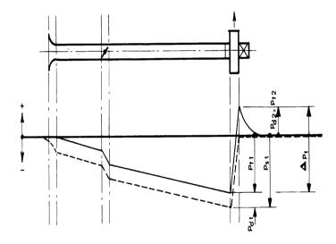
$$\Delta p_{\text{total system}} = \Delta p_{\text{static system}} = p_{\text{total fan}}$$
