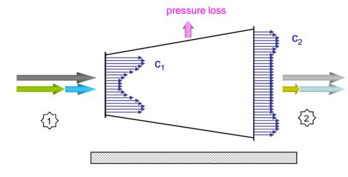
Downstream of a fan the velocities are not uniform. Standard literature to calculate the diffuser efficiency is not 100% accurate.
